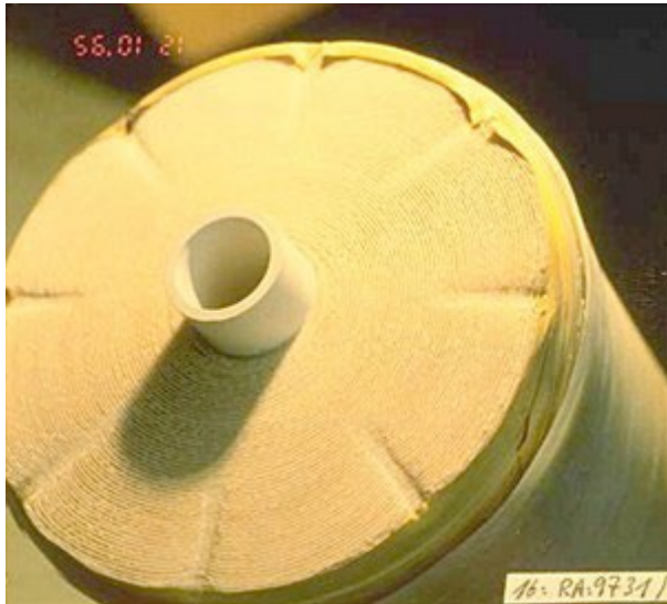
Figure 59: The endcap has been pushed off
