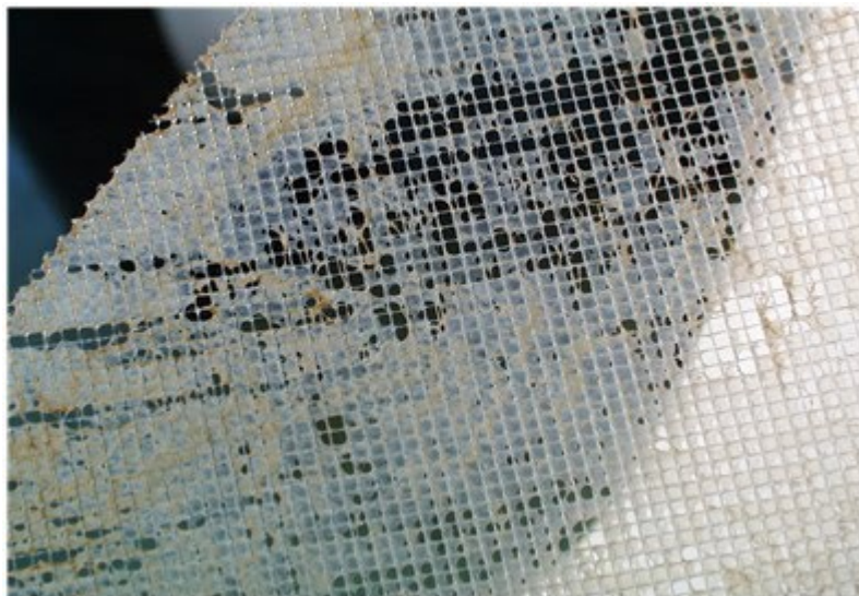
Figure 55: Picture of feed spacer with biofilm
